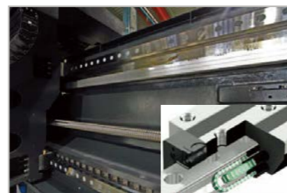
Ultra loading roller type linear guideways on X & Y axes.
