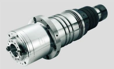
Belt type spindle has an advanced labyrinth structure that can avoid coolant from getting into inside of the spindle unit and increase the durability of the spindle. A spindle air blast device automatically clean the interior part of the spindle taper during tools change
