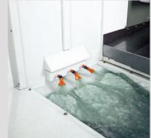
The coolant through spindle device gives 10 or 20 bars high pressure cooling effect. The coolant passes through the spindle and flushes through the tool edge for directly cooling the workpiece and tool edge.
