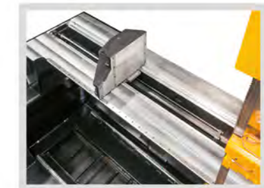
Clamping Vise Strong and hydraulic clamping vise holds the workpiece firmly during cutting.
