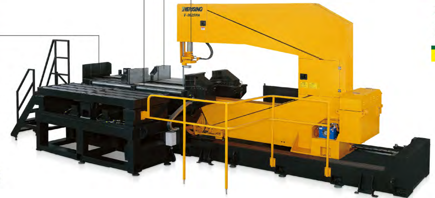
Guide Arm Guide arm is hydraulically operated.
