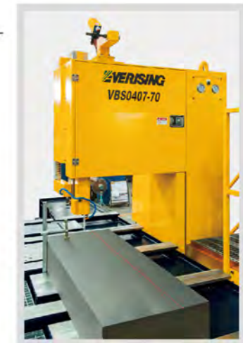
Laser Projector (Optional) By using the laser projector for making line prior to cutting, more accurate size of cut can be ensured.
