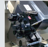
VDI 40 Driven tool system VDI 40動力刀塔
