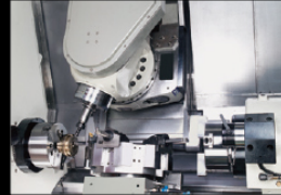
Mill/Turn by B-axis tool spindle
