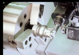
Belt driven spindle available with C axis
