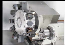
Built-in spindle available with C/Y axes & Subspindle
