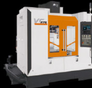
Belt driven spindle up to 10000 rpm Box slideways available
