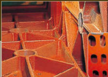
Cross-diagonal ribbing in column to prevent flexing during machine operation.
