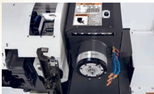
Arm type ATC + Coolant ring + LED lights
