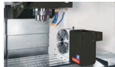
4 th axis interface for rotary table
