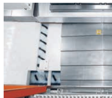
Bottom guarding flush + Screw chip removers
