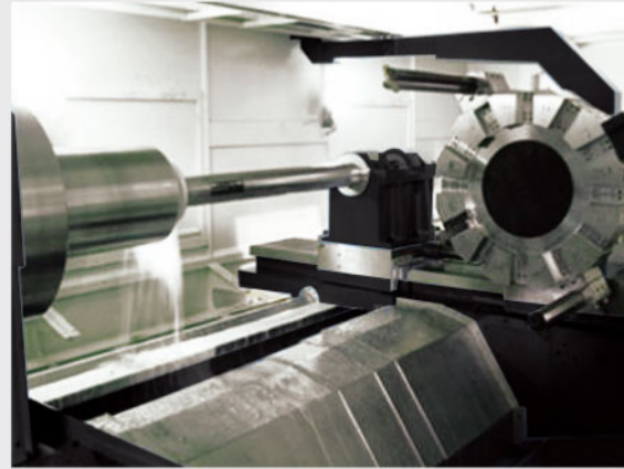
Deep Hole Boring
